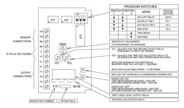
WHEN USED WITH THE "E" SERIES FEEDER CONTROLS, THE THREE POTENTIOMETERS FOR SENSITIVITY AND TIMING ARE ACCESSIBLE BY REMOVING THE BLACK PLUG IN THE FACE PLATE. CAREFULLY ADJUST THE APPROPRIATE POTENTIOMETER WITH AN INSULATED SCREWDRIVER.
