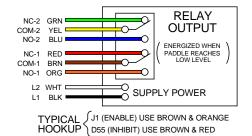
WARNING: Black lead must be connected to FUSED power.
